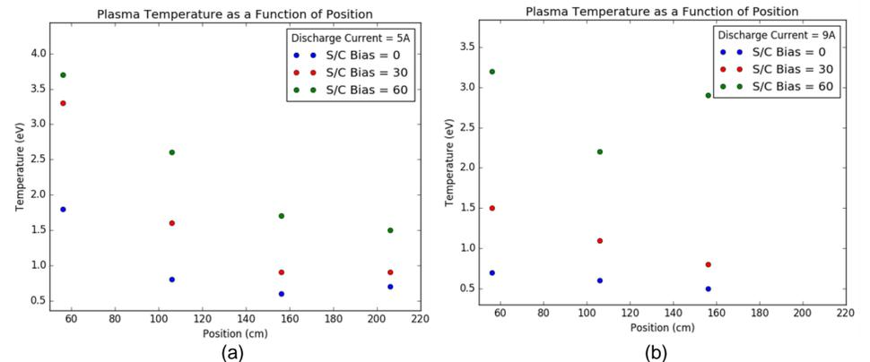
Figure 5: Electron temperature as a function of distance downstream for of (a) 5 and (b) 9A. The electron temperature increases with spacecraft bias and decreases with increasing distance relative to the hollow cathode.
