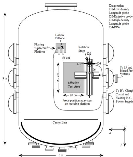
Figure 1: Experimental setup within PEPL's LVTF.
