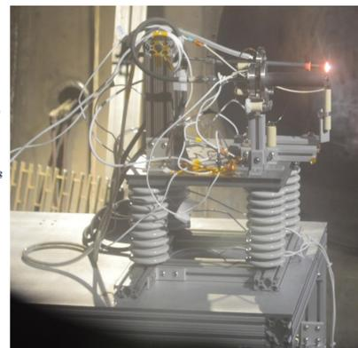
Figure 2: Electrically isolated conducting platform and hollow cathode.
