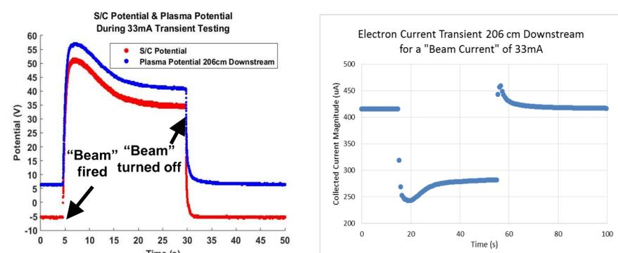
Figure 4: Plasma potential, spacecraft bias, and electron current for a current of 33 mA and 5A discharge current. The electron flux and plasma potential trace the S/C potential.
