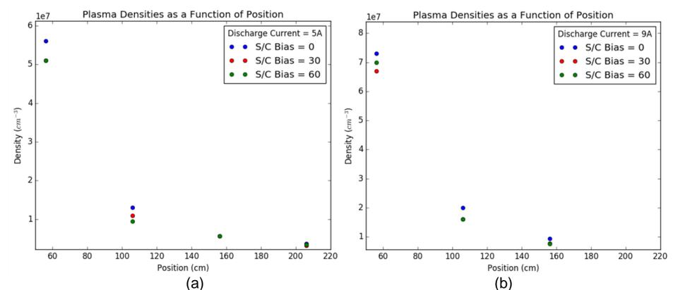
Figure 6: Plasma density as a function of distance downstream for discharge currents of (a) 5 and (b) 9A. The density does not seem dependant on spacecraft bias as the values are roughly constant as the spacecraft bias changes. However, it decreases with increasing distance relative to the hollow cathode.
