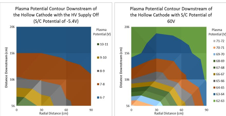
Figure 3: Plasma potential contour maps for spacecraft biases of 0 and 60 V for a discharge current of 5A. The potential drop across the plasma increases with S/C bias.
