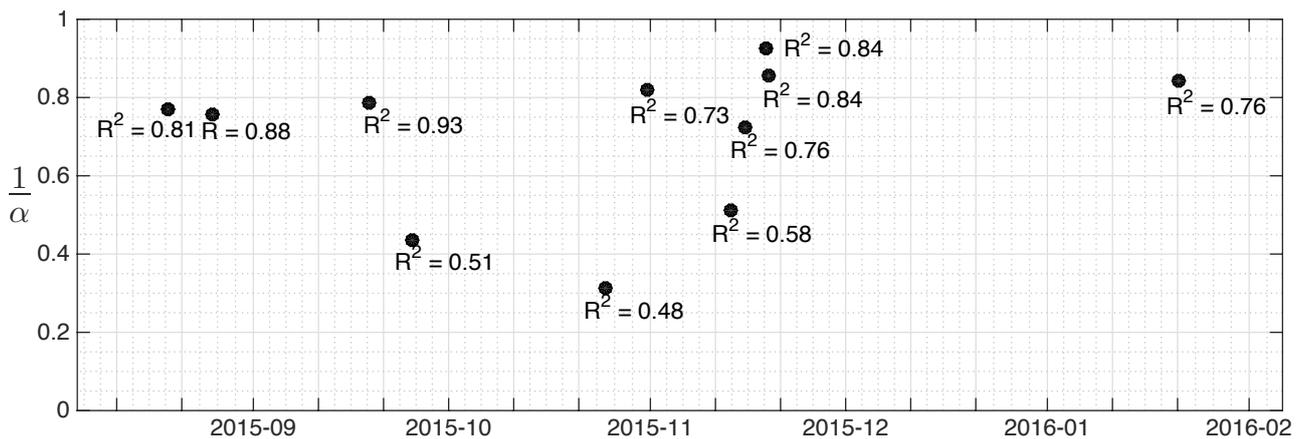
Figure 3. Overview of the fraction  $1/\alpha$  of  $V_{float}$  picked up by LAP1 annotated with the  $R^2$  coefficient of determination between  $V_{float}$  and  $E_{ion,threshold}$  for each measurement block.
