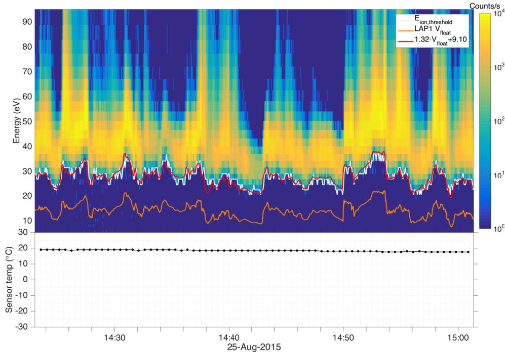
Figure 1. ICA high time resolution ion energy spectra under stable sensor temperature. LAP1 spacecraft potential measurements (orange line) correlate well with the ion threshold energies (white line). Also shown: LAP1 spacecraft potential measurements corrected by a factor of 1.32 and with an offset of 9.1 V (red line).
