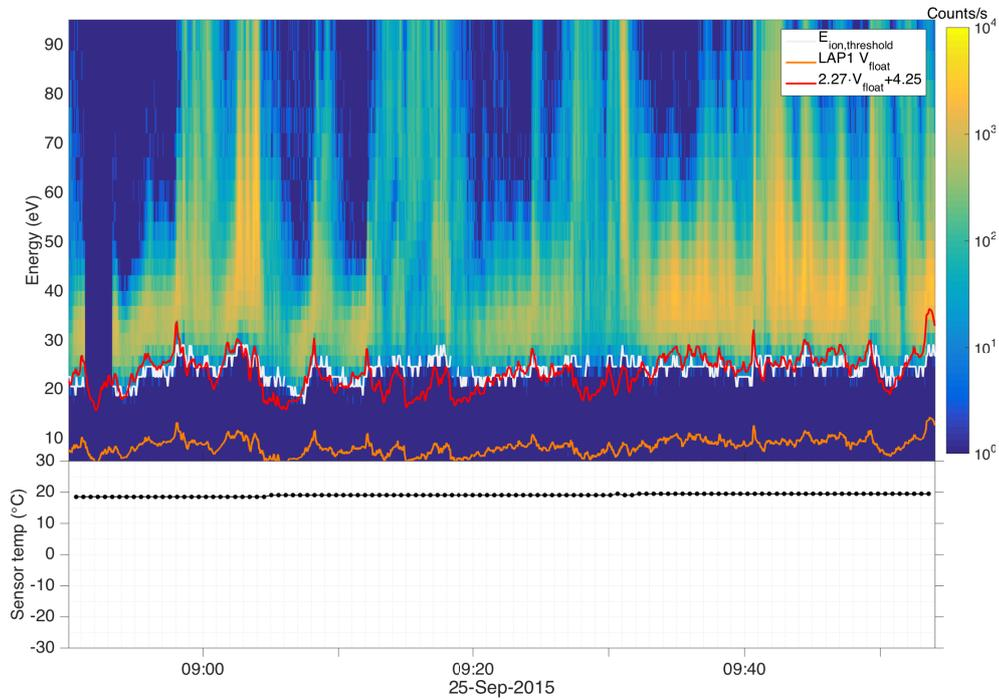
Figure 2. ICA high time resolution ion energy spectra under stable sensor temperature but intermittently subdued local ionization. The correlation between LAP1 spacecraft potential measurements (orange line) and the ion threshold energies (white line) is lost during periods of weak ion flux.
