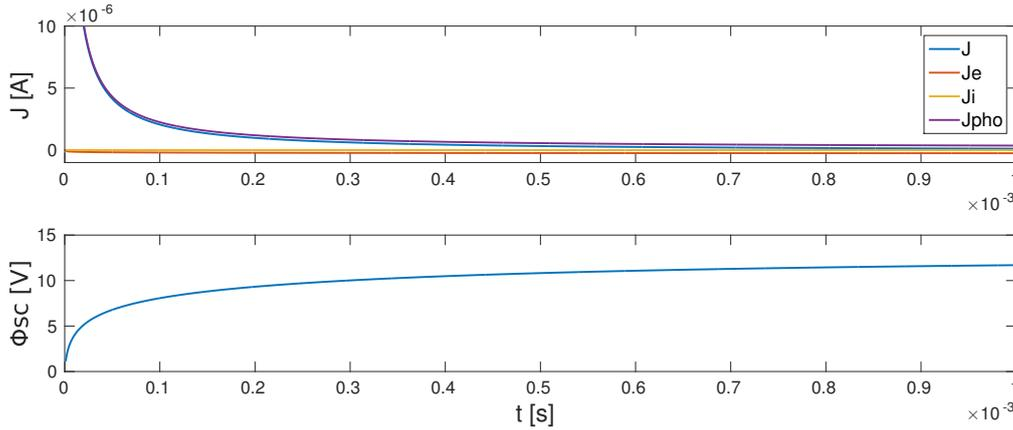
Figure 1. The temporal evolution of all charging currents (top) and the spacecraft potential (bottom) for density of electrons and ions  $n = n_e = n_i = 0.1 \text{ cm}^{-3}$  and plasma temperature  $T = T_e = T_i = 5 \text{ eV}$
