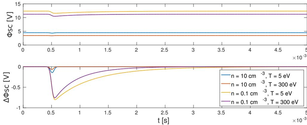
Figure 3. The temporal evolution of the spacecraft potential (top) and change in the equilibrium potential (bottom) during dust impact for various plasma environments.
