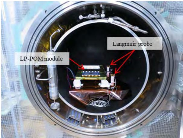
Fig.2.2-1 LP-POM inside the vacuum chamber
