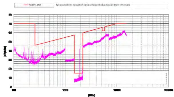
Fig.3.2-4 Radio emission due to electron emission
