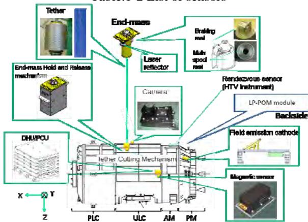
Fig.1-3 The components on HTV
