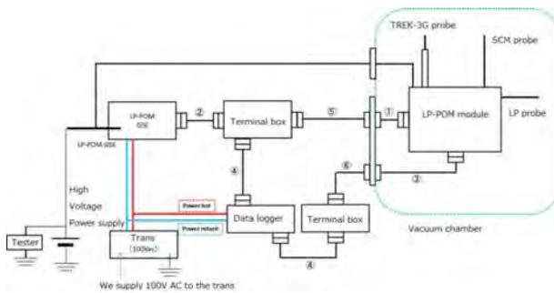
Fig.2.2-2 Block diagram of experiment system
