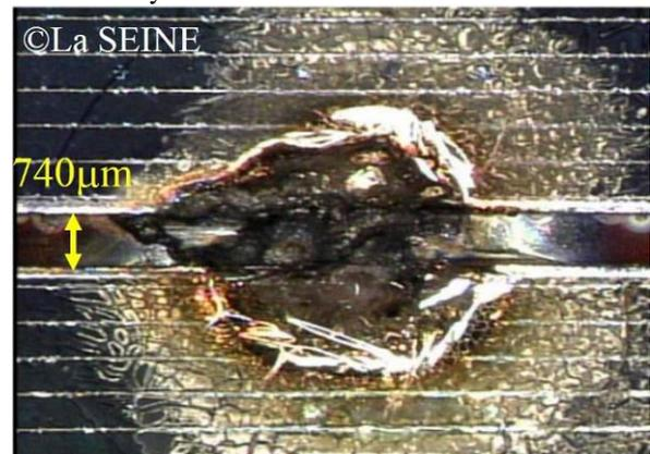
Fig.2. Permanent Sustained Arc Crater
