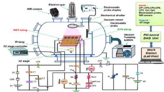
Figure2 Circuit for GEO secondary arcing experiment
