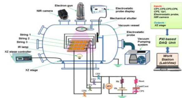
Fig 1 Experimental Setup for primary experiments
