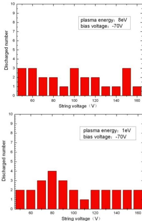
Figure 5. Arc discharge numbers of high-voltage solar array in different energy plasma
