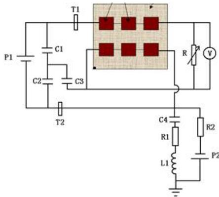
Figure 2. Schematic diagram of high voltage solar array simulation circuit
