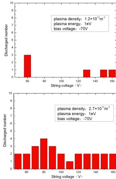
Figure 6. Arc discharge numbers of high-voltage solar array in different density plasma
