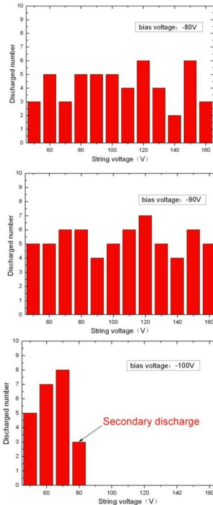
Figure 3. Discharged numbers of high-voltage solar array depended on string voltage when bias voltage is -70V, -80V, -90V and -100V relatively
