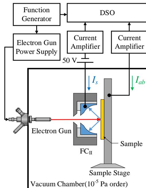
Figure 1. Measurement system
