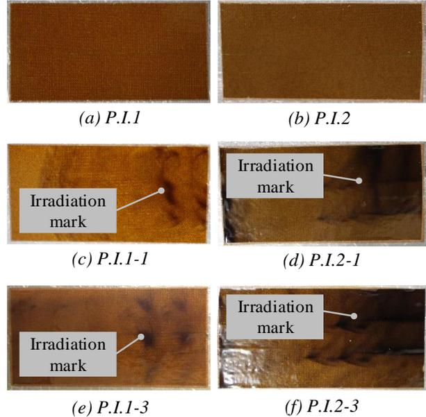
Figure 3. Appearances of P.I.1 (left line) and P.I.2 (right line) before and after irradiated electron beam
