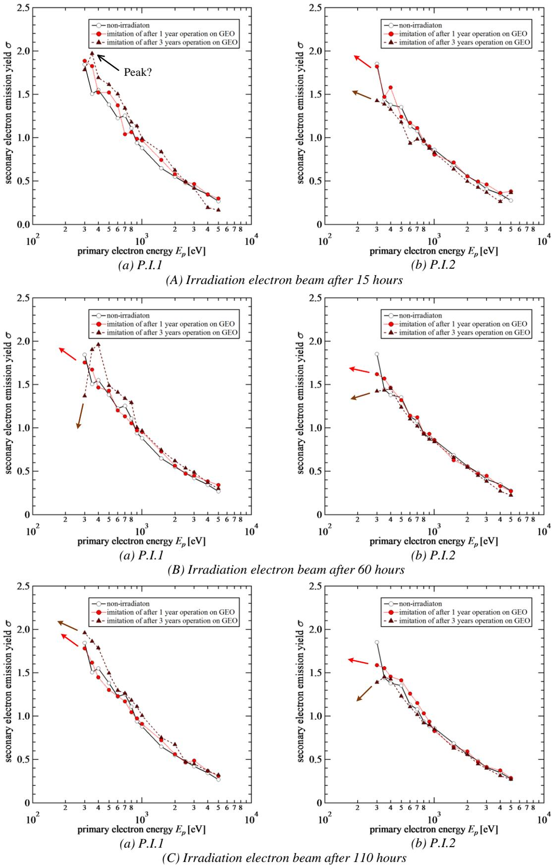
Figure 6. The change of SEEY by electron beam irradiation dose of P.I.1 (left line) and P.I.2 (right line)
