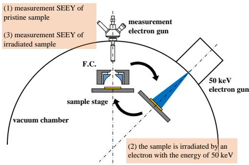
Figure 2. Electron beam irradiation system
