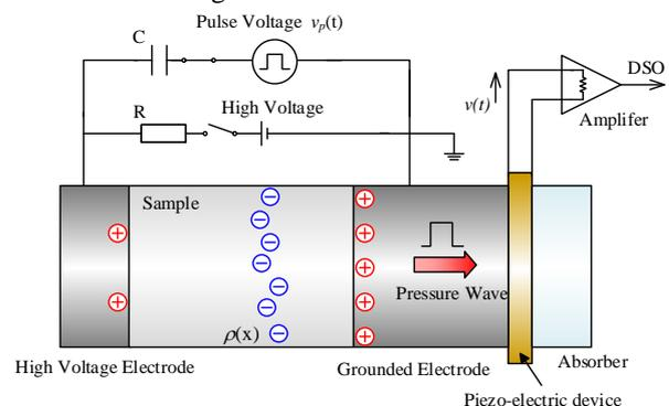
Figure 1. Schematic view of PEA measurement method
