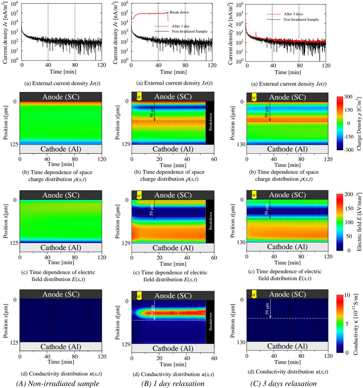
Figure 4. Measurement results of non-irradiated and irradiated PI-2 under DC stress
