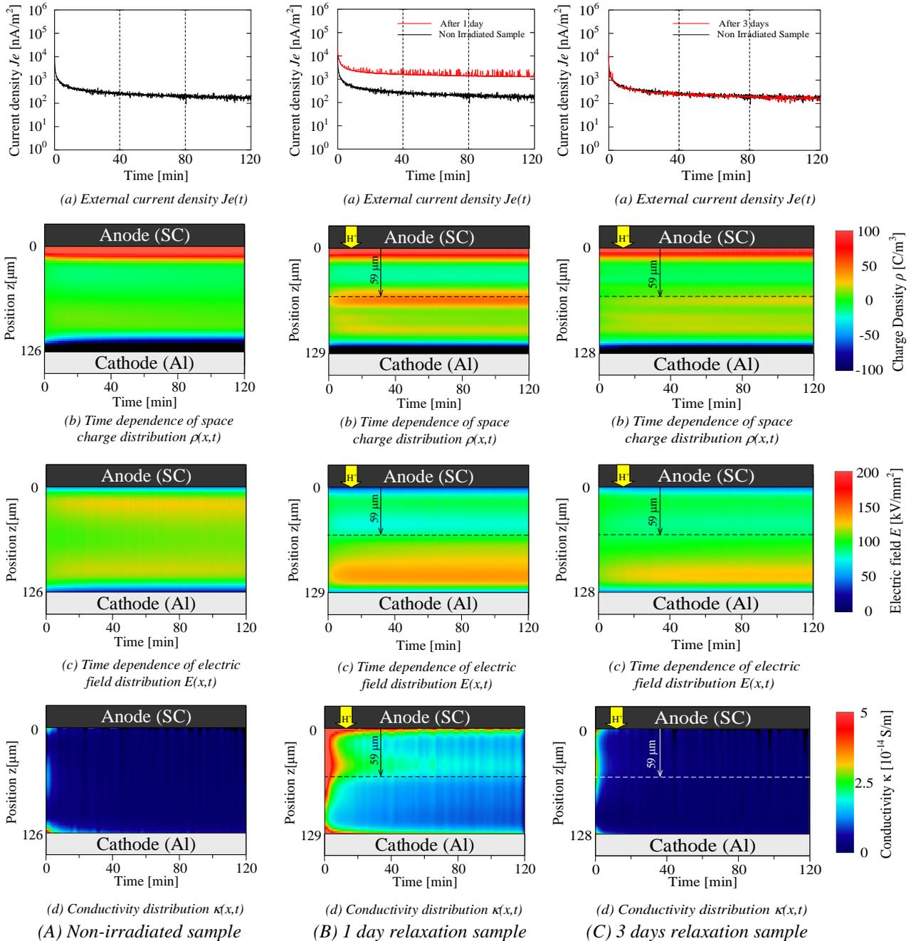
Figure 3. Measurement results of non-irradiated and irradiated PI-1 under DC stress
