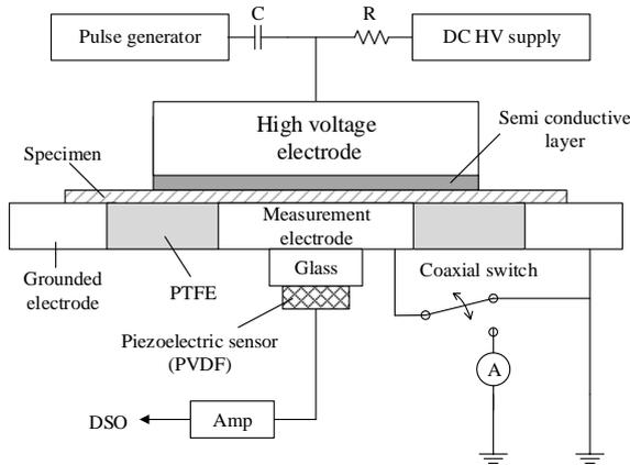
Figure 2. Schematic view of space charge distribution and conduction current simultaneous measurement system
