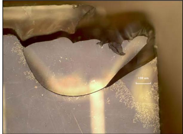
Fig. 2. Lichtenberg-like figuring of an arced coverglass corner.
