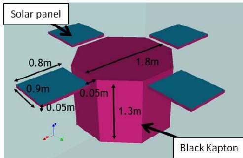
Figure 4. The charging simulation model of the Van Allen Probes.
