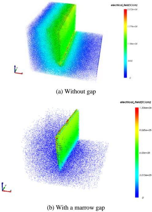
Figure 5. Distribution of electric field in structure A
