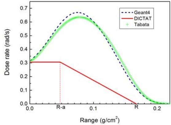
Figure 2. Dose rate as a function of depth in polyimide for a normally incident 0.5 MeV electron beam
