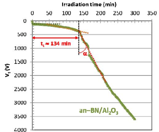
Figure 3. Temporal evolution of the surface potential of an-BN/Al<sub>2</sub>O<sub>3</sub> under critical irradiation (20 keV, 750 nA.cm<sup>-2</sup>, T°C room, focused beam)[4]
