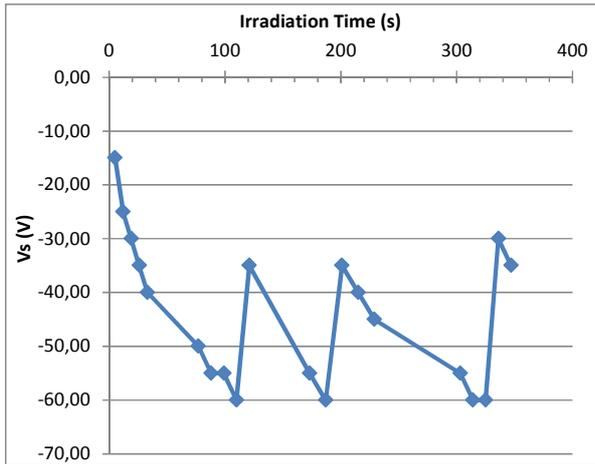
Figure 2. Evolution of surface potential measured with the REPA method on an-BN/Al<sub>2</sub>O<sub>3</sub> irradiated at 10 keV and 1 nA.cm<sup>-2</sup>
