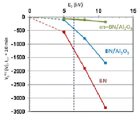
Figure 1. Evolution of the equilibrium surface potential (measured with the KP method) of BN, BN/Al<sub>2</sub>O<sub>3</sub> and an-BN/Al<sub>2</sub>O<sub>3</sub>, as a function of the incident energy after 10 min under electron irradiation (10 nA.cm<sup>-2</sup>, room temperature, defocused beam)[4]
