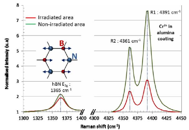
Figure 4. Raman spectra measured at 532 nm incident wavelength on pristine and aged an-BN/Al<sub>2</sub>O<sub>3</sub>
