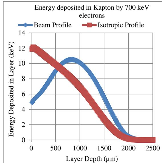
Figure 2: Electron energy deposition profile, 700 keV
