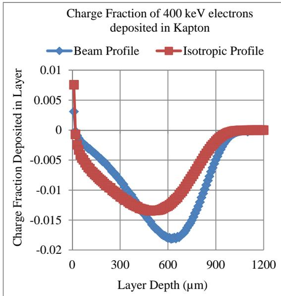
Figure 7: Charge Fraction profiles for 400 keV
