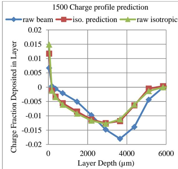
Figure 10: Charge fraction profiles for 1500 keV
