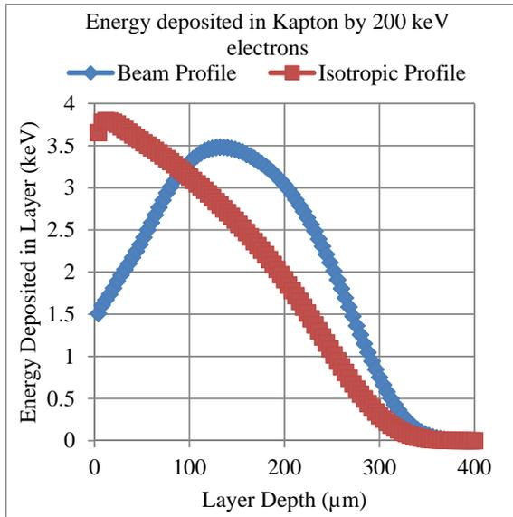
Figure 1: Electron energy deposition profile, 200 keV
