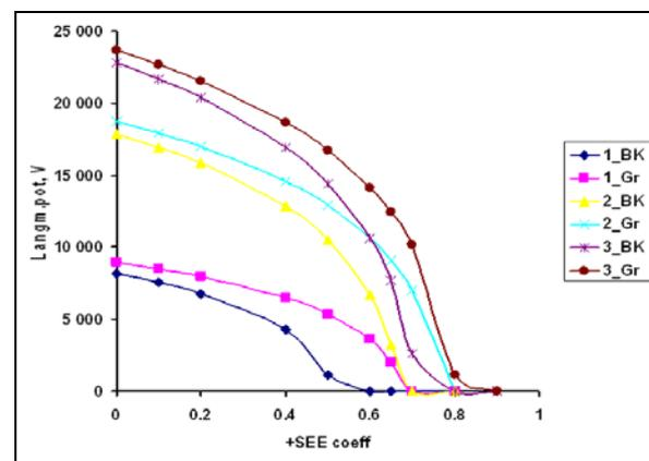
Figure 4. Potential values vs SEE coefficient variations for spacecraft charging in hot plasma with following parameters:
