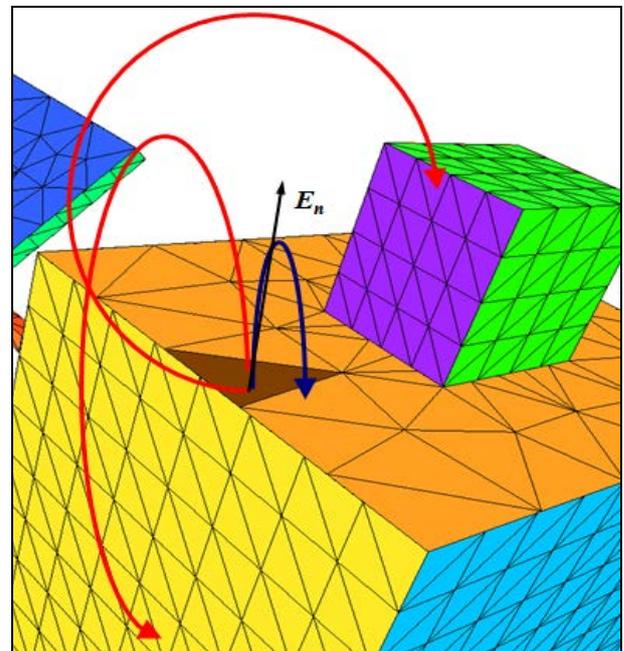
Figure 1. Examples of the secondary electron trajectories in the vicinity of the charged spacecraft
