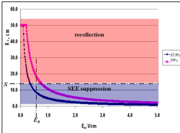
Figure 3. Recollection radius vs electrostatic value on the discrete surface element
