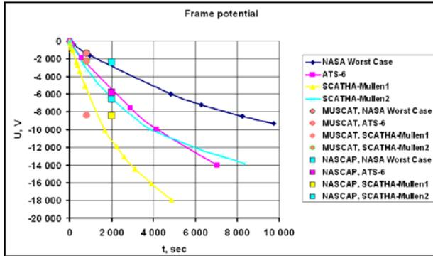
Figure 5. Electric potential of the spacecraft metal frame in the various charging cases
