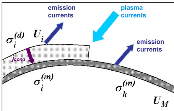
Figure 2. Spacecraft charging electrostatics
