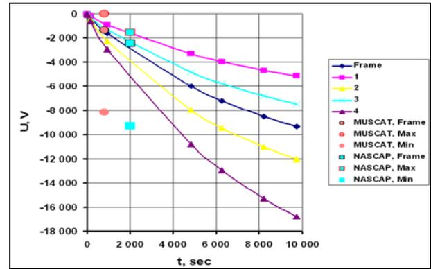
Figure 3. Electric potential of various spacecraft elements vs charging time compared with NASCAP and MUSCAT results [2] in the NASA Worst Case
