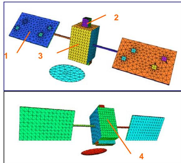
Figure 1. NASCAP spacecraft model. Electric potentials in points 1 – 4 as function of the charging time is shown in Results section
