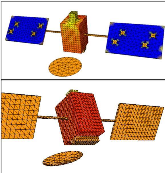
Figure 6. Stationary potential distribution in the ATS-6 case
