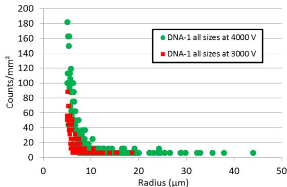
Figure 4: Dust size distributions of contamination observed at 3000 and 4000 V
