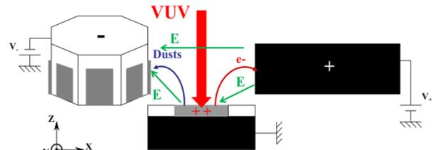
Figure 3: Experimental configuration inside DROP
