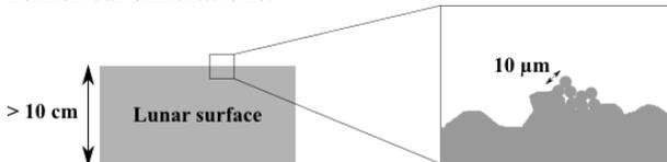
Figure 1: (left) Representation of a dust layer at a macroscopic scale. The zoomed box represents the dust layer surface at a microscopic scale, taking account of the microscopic irregularities and tips effects.
