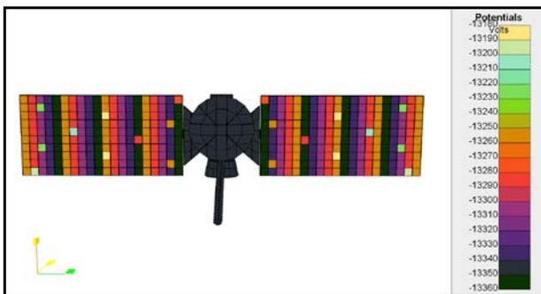
**Figure 2: Simulated spacecraft surface potentials for the 15 R<sub>J</sub> worst case auroral environment.**
