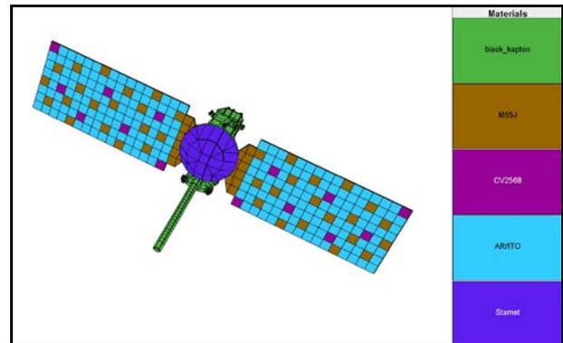
**Figure 1: Geometrical model of the Europa spacecraft in *Nascap-2k* Object Toolkit.**
