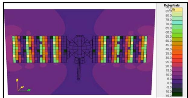
**Figure 4: Simulated spacecraft surface potentials for the warm near-Europa (torus) environment.**
