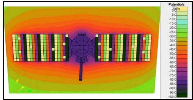
**Figure 3: Simulated spacecraft surface potentials for the cold near-Europa (ionosphere) environment.**
