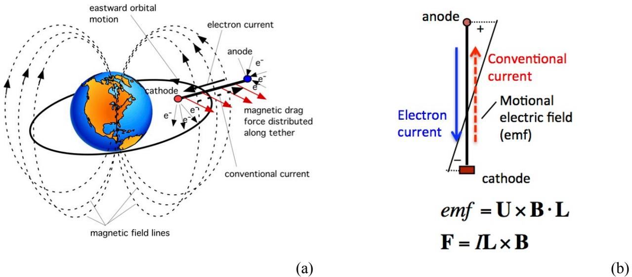
**Fig. 1** (a) electrodynamic tether with anodic and cathodic terminations, and (b) schematic of motional electric field  $emf$  and Lorentz force  $F$  with tether current  $I$ , orbital velocity  $U$ , magnetic field  $B$ , and tether length  $L$ .
