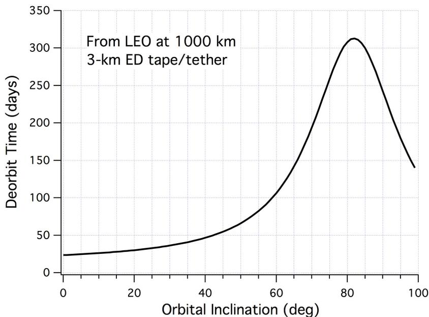
**Fig. 3** Deorbiting time vs. orbital inclination for a tethered system with a 3-km  $\times$  25-mm EDT attached to a 1000 kg satellite from a 1000-km orbit through reentry for average solar activity
