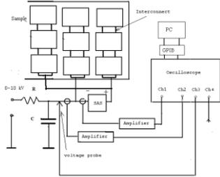
Figure 3. Circuitry diagram for registering primary ESDs and sustained arcs
