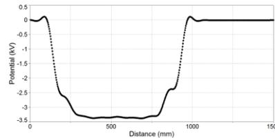
Figure 6. Surface potential is shown after 20 minutes irradiation with electron beam.
