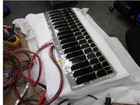
Figure 1. Test coupon with fully encapsulated all dielectric-conductor junctions.
