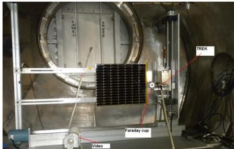
Figure 13. Coupon is shown mounted inside chamber.
