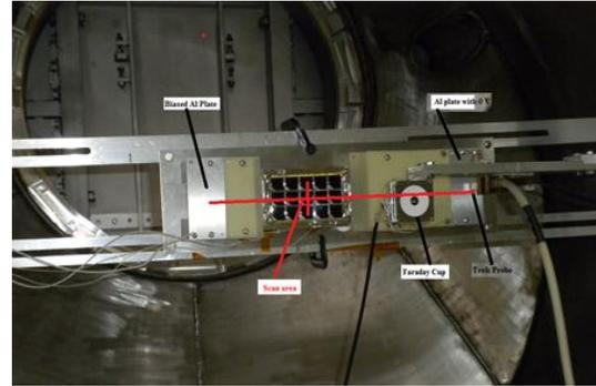
Figure 16. Setup for surface potential measurements.
