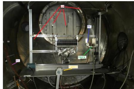
Figure 2. Coupon and diagnostic equipment are shown inside vacuum chamber.
