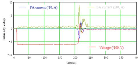
Figure 12. One example of pulses for SA test: bias-600 V, PA peak -40 A, SAS current peak 0.8 A.
