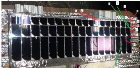
Figure 7. Arc sites are shown for test at 175 C (red), and for test at 9 C (green).
