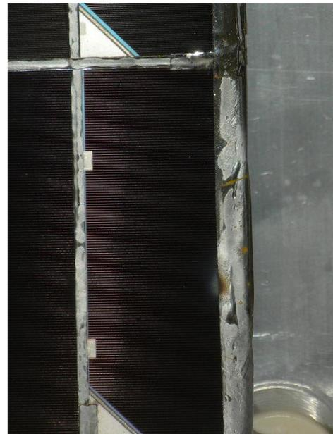
Figure 10. Visible trace of arc was found on edge of foil.
