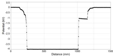
Figure 5. Surface potential is shown for biased sample before irradiation
