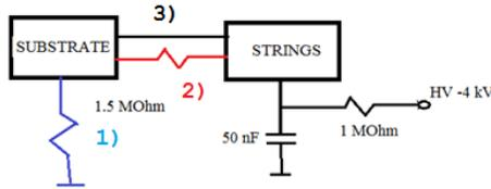
Figure 9. Three different circuitry diagrams that were used in GEO arcing tests.
