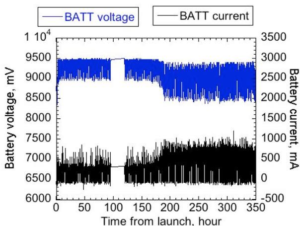
Figure 6 HORYU-IV battery condition for the first two weeks
