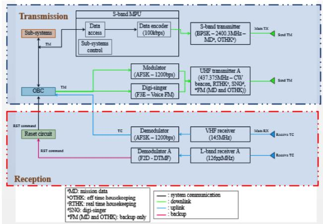
Figure 2 AEGIS communication block diagram
