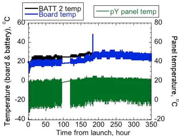
Figure 5 HORYU-IV temperature for the first two weeks
