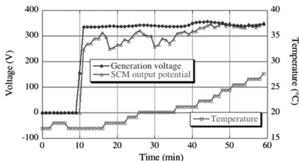
Figure 3 HORYU-II on orbit data of HVSA mission [2]
