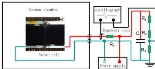
Fig.9.The setup for the experiment
