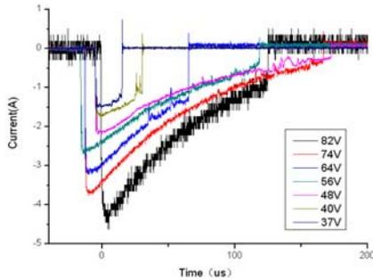
Fig.13.The discharge current change with voltage
