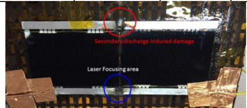
Fig.15.The soar array after experiment
