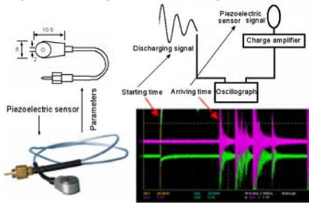
Fig.2. Particles velocity measured by piezoelectric sensor.
