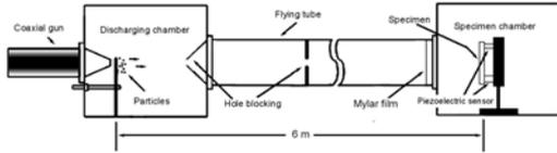
Fig. 1. Sketch map of plasma drag particles accelerator
