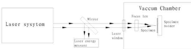
Fig.3.The composition of laser inducing plasma system
