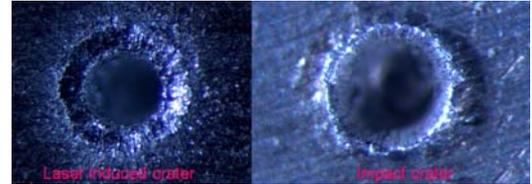
Fig.4. The craters on aluminum plate
