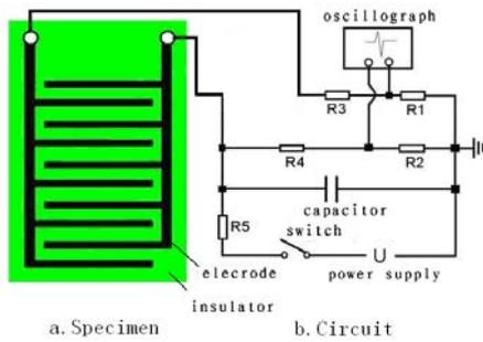
Fig7.The specimen and the circuit for the experiment
