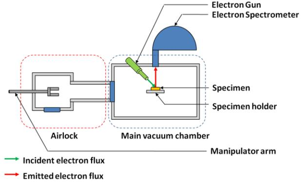
Figure 5 DEESSE test-bed scheme (DESP, ONERA)
