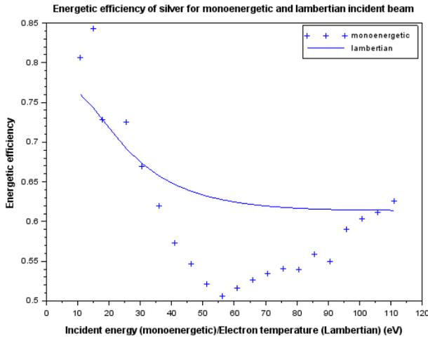
Figure 6 Silver energetic efficiency of plasma/wall interaction
