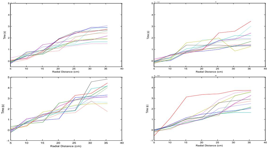
Figure 5: Peak current time vs. electrode radius for multiple flashover events on Al-BB (top left), Al-250P (top right), Ta-BB (bottom-left), and Ta-250P (bottom-right)
