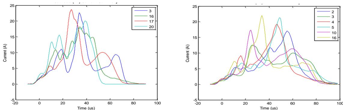
Figure 7: Discharge (R1) waveforms with 100nF external capacitance for multiple flashover events on Al-BB (left), and Ta-BB (right)
