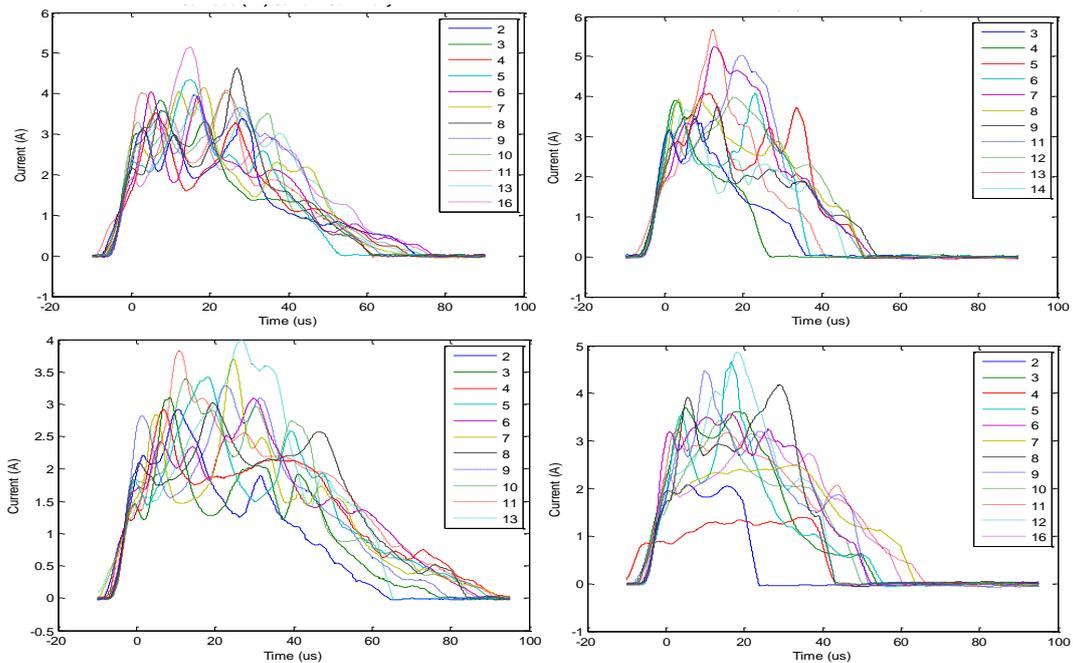
Figure 4: Discharge (RI) waveforms for multiple flashover events on Al-BB (top left), Al-250P (top right), Ta-BB (bottom-left), and Ta-250P (bottom-right)
