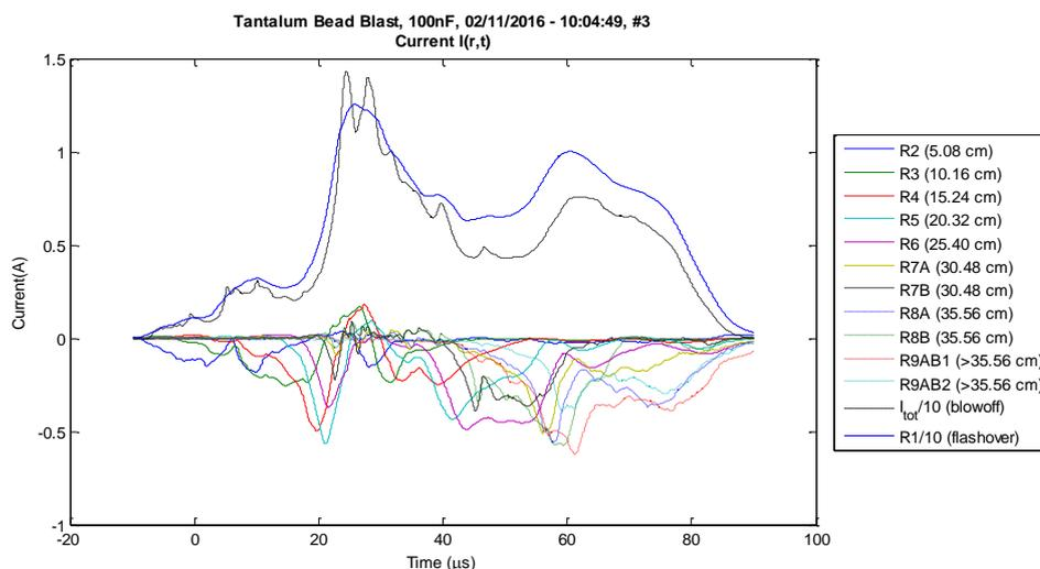
Figure 6: Typical discharge for bead-blasted Tantalum with 100nF external capacitance
