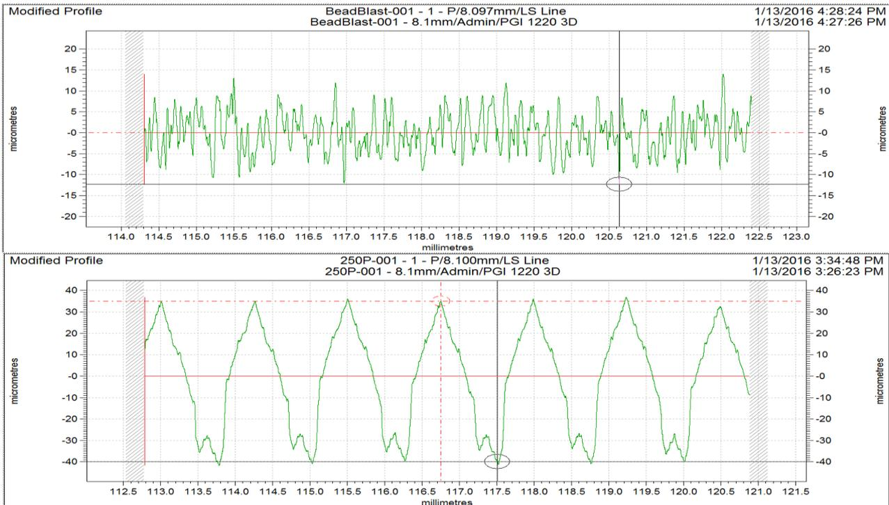
Figure 3: Surface profiles of bead-blast (top) and 250P mill (bottom) finishes on Aluminium
