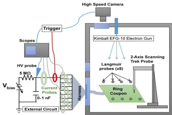
Figure 1: Apparatus for IG ESD testing
