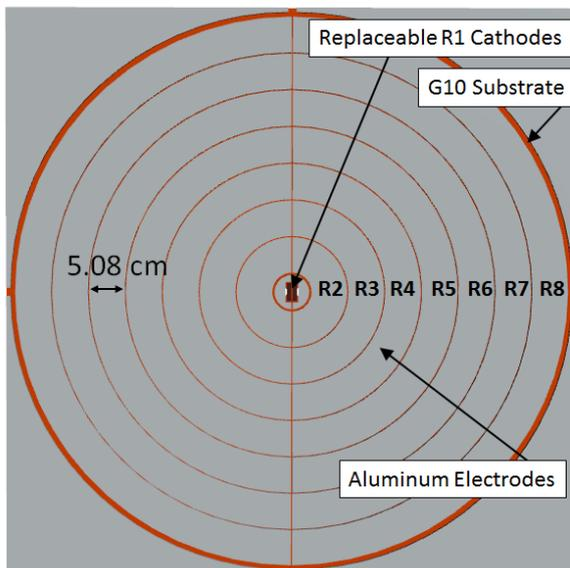
Figure 2: Diagram of Annular electrode test article
