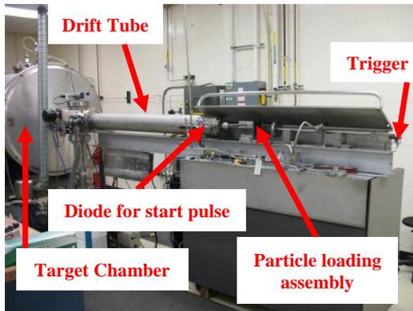
Figure 2. Side View of the Micro Light Gas Gun at the NASA MSFC Impact Test Facility
