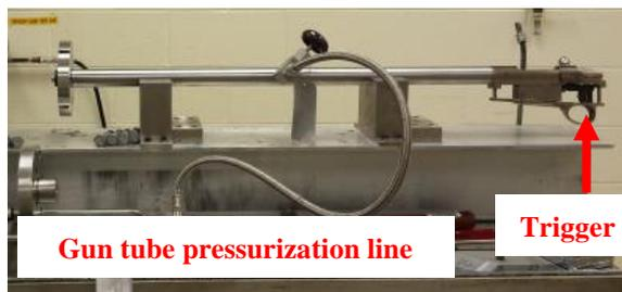
Figure 3. Close-up view of firing line.
