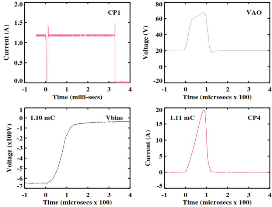
Figure 11. Current and voltage probe data for impact 2B. CP1 shows SAS current flow and is stopped by the arc interruption circuit at ~ 3 milli-sec. The charge contained in the primary arc is calculated via two methods and is noted on the Vbias and CP4 panels. A small difference in primary arc amplitude and duration is noted between the proxy coupon with copper plates and Coupon A.
