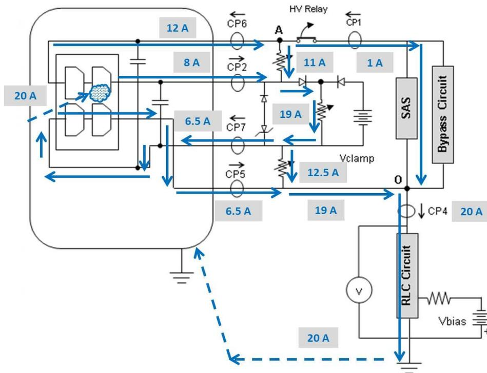
Figure 14. Diagram of paths for primary arc current during impact 2B.
