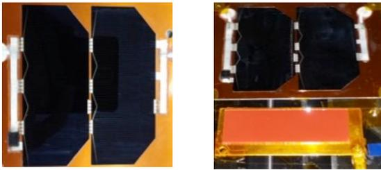
Figure 15. Horyu IV FM solar cell coupon (left) and charging test setup in vacuum chamber (right)
