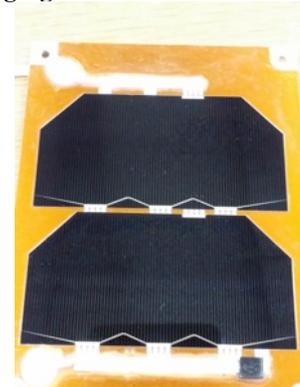
Figure 7. ATO coating solar cell sample (for Horyu IV EM)
