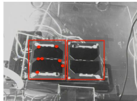
Figure 10. Arcing occurred on non-coated solar cell (left). No arcing occurred on coated solar cell (right)
