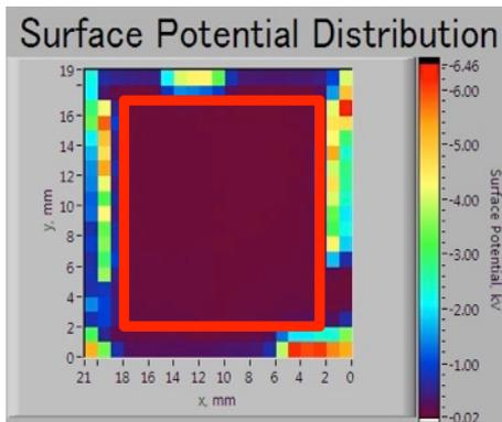
Figure 8. Charging test result on Horyu IV EM solar cell at 10 keV
