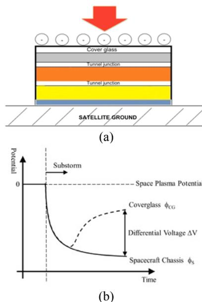
Figure 1. Charging and arcing mechanism on solar cell.
