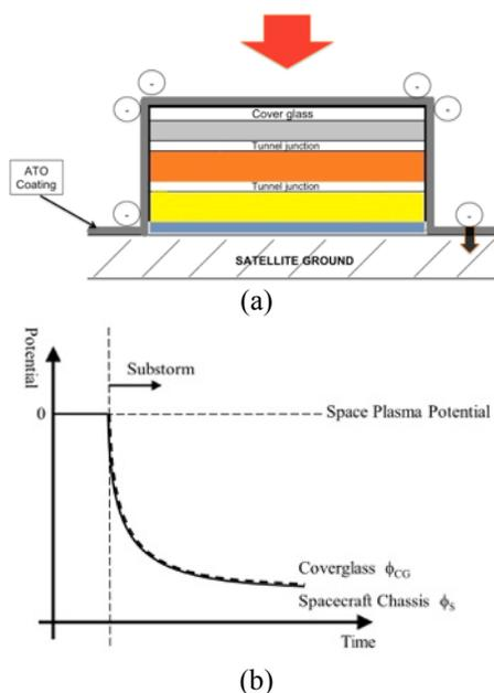
Figure 2. Charging and arcing mitigation mechanism due to ATO coating. (a) Cross sectional view of solar cell with coating. (b) Surface potential on solar cell with coating<sup>[3]</sup>.
