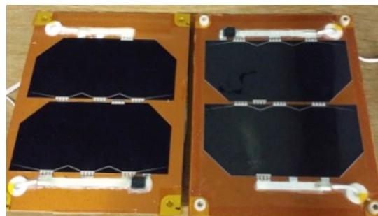
Figure 4. Coated (right) and non-coated (left) solar cell
