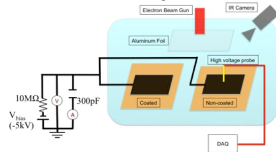
Figure 9. Arcing test setup
