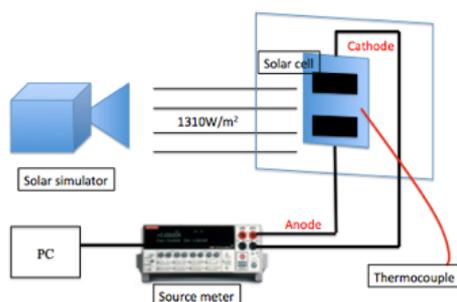
Figure 13. Setup of current-voltage characteristic measurement.
