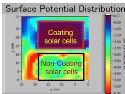
Figure 12. Charging test result on Horyu IV EM solar cell after thermal cycling at 10keV
