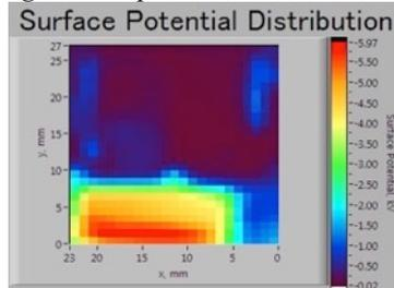
Figure 16. Charging test result on Horyu IV FM solar cell at 10 keV
