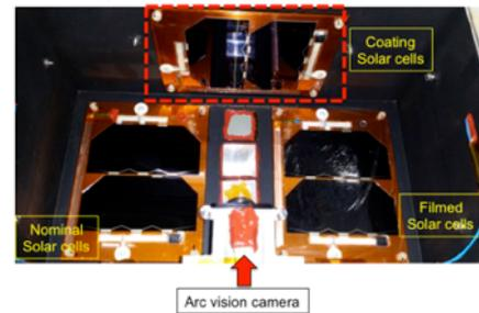
Figure 17. ATO coating solar cell coupon mounted on Horyu IV satellite (flight model)
