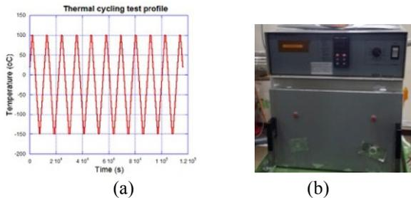
Figure 11. Thermal cycle temperature profile (a) and Depatch 900 machine (b).
