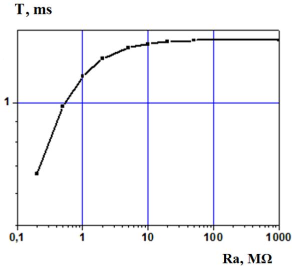
Figure 3. The dependence of the oscillation period from  $R_a$
