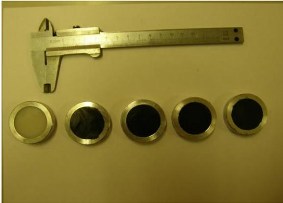
Figure 6. Samples for test on the resistance to ESD occurrence
