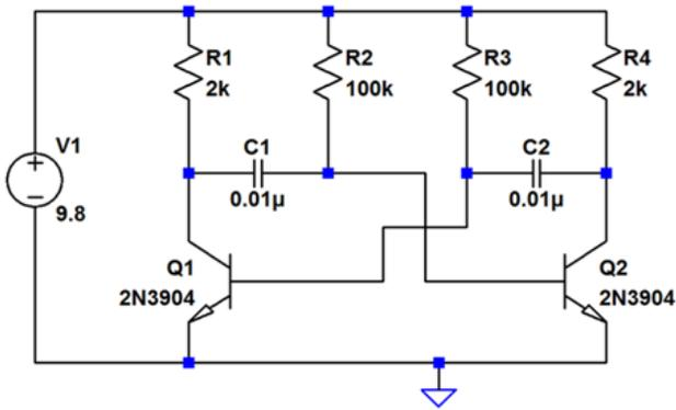
Figure 1. Basic multivibrator electric diagram.
