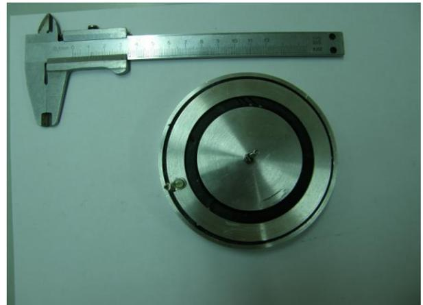
Figure 5. Sample with model dielectric for conductivity measurements
