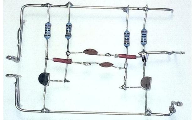
Figure 4. The multivibrator skeleton- mode mock-up
