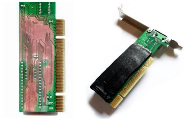
Figure 7. The network card without a layer of protective resin on the left and covered with a layer of nanoconductive dielectric on the right
