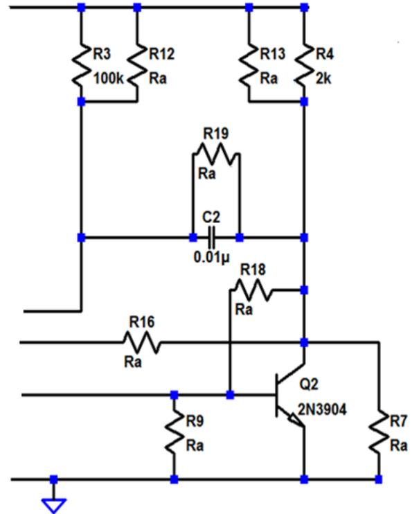
Figure 2. Fragment of the multivibrator circuit with additional resistors with value of  $R_a$
