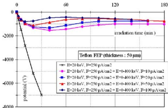
Figure 2 Laboratory measurements of Teflon charging [2] due to a 20keV electron beam with and without high energy electrons.
