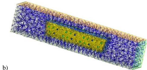
Figure 6: a) geometrical model and b) mesh of the 25 pins D-Type connector.
