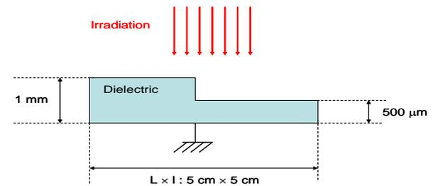
Figure 1: Schematic representation of the step geometry.
