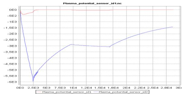
Figure 4: Simulation results of surface potential evolution with irradiation at 350 keV on PTFE step sample
