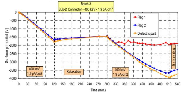
Figure 7: Evolution of surface potential during the test performed on 25 pins d-type connector
