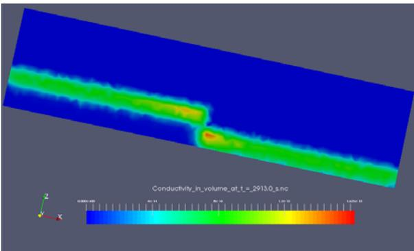
Figure 5: Conductivity map in the dielectric at  $t = 2900s$  and energy of  $350keV$
