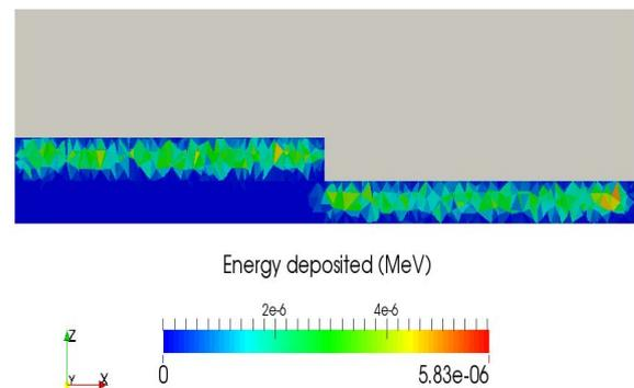
Figure 2: Dose deposited in MeV by incident  $e^-$  at 0.35 MeV (calculation from Geant4/GRAS).
