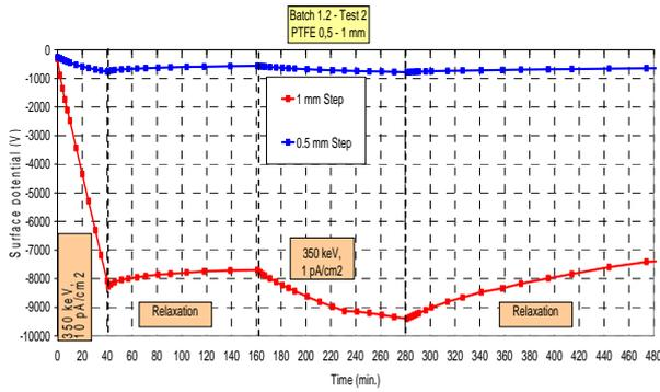
Figure 3: Measurement of surface potential evolution with irradiation at 350 keV on PTFE step sample
