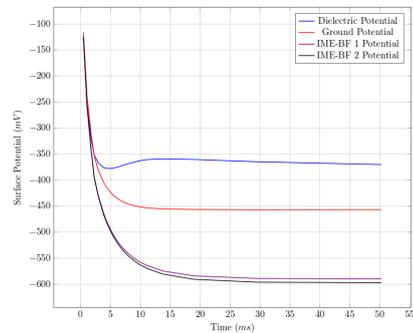
Figure 5: Temporal variation of the surface potentials using the coupled method for ions O+
