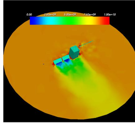
Figure 3: Ionic density of O+ ( $m^{-3}$ ) using the coupled method for ions
