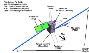
Figure 1: Geometry and Materials used on SPIS simulations
