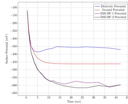
Figure 4: Temporal variation of the surface potentials using a PIC distribution for ions O+
