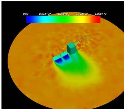
Figure 2: Ionic density of O+ ( $m^{-3}$ ) using a PIC distribution for ions
