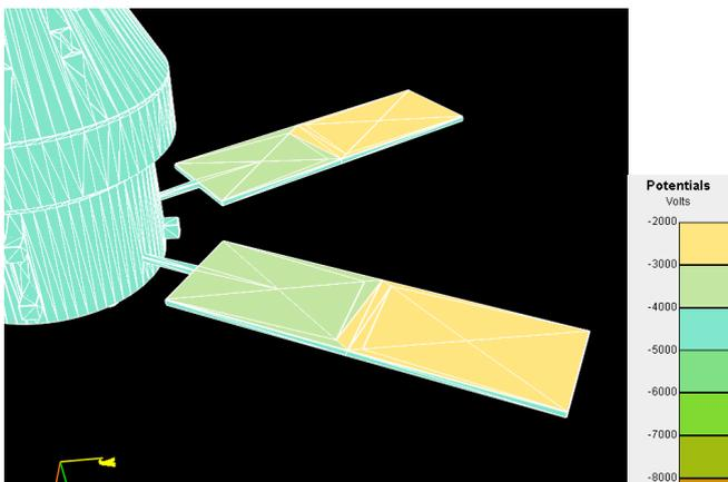
Figure 5: A three dimensional color plot of the induced voltage on the high resolution DELC mesh at the end of the simulation. We have focused in on the solar panel since that is where the maximum voltage is occurring.
