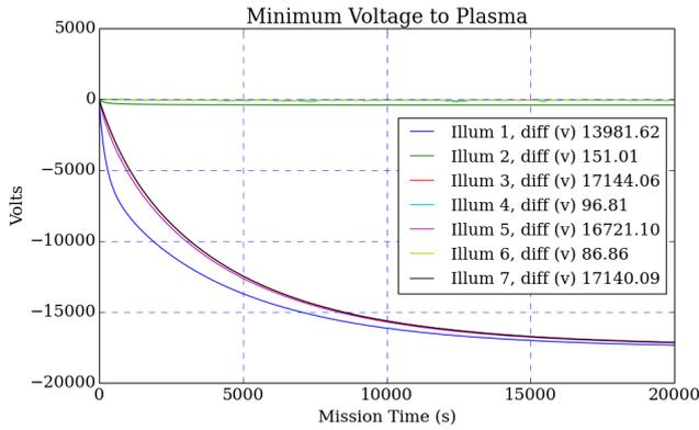
Figure 3: The plot shows the minimum voltage induced on the vehicle as a function of time for each illumination scenario. The value next to *diff* refers to the difference between the minimum and maximum voltage seen on the vehicle at the end time - not differential voltage in terms of neighboring surfaces. See text for details.
