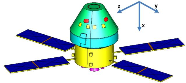
Figure 1: The Orion-like spacecraft used in this analysis and described in section 3. The depiction is the CAD based model used for development of the geometry. Colors represent different material regions. See the text for more information.
