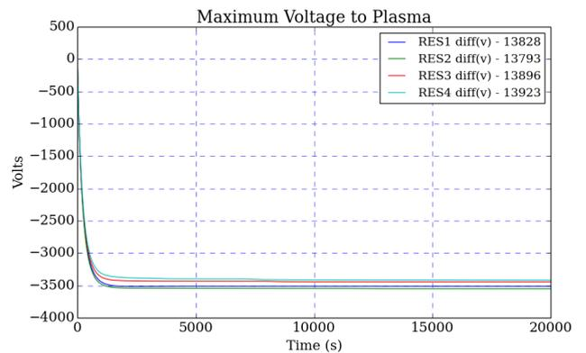
Figure 6: The maximum voltage as a function of time for four different resolutions of the DELM mesh. The resolutions range from RES1 to RES4: 2136, 1762, 1584 and 1208 elements.
