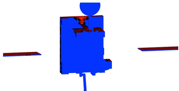
Figure 6. Purely specular reflection from dish onto surface of spacecraft bus with  $+15^\circ$  incidence
