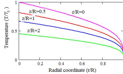
Figure 5. Electron temperature spatial distribution.
