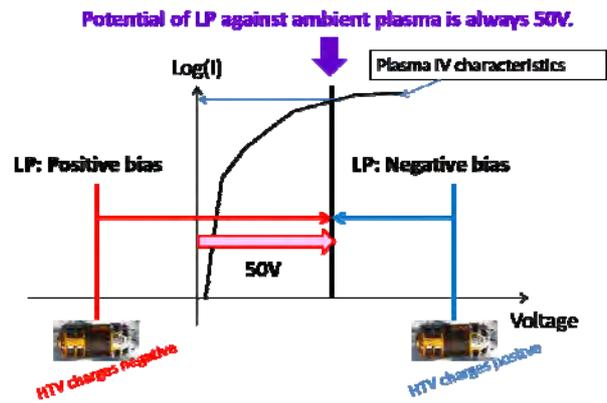
Fig.2-2 Mechanism of LP of KASPER module
