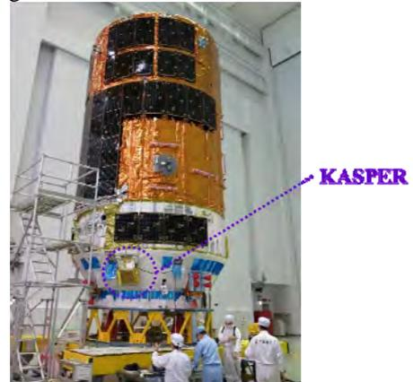
Fig.2-3 The position of KASPER module on HTV-5
