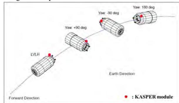
Fig.2-4 The relationship between the position of KASPER module and the attitude of HTV-5
