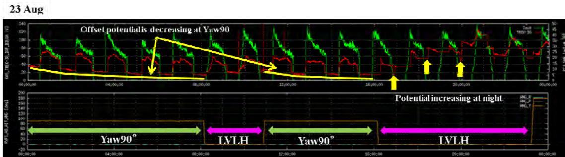
Fig.3.2-3 The data at 23 August: Upper graph shows solar array output current (Green line) and potential of HTV (Red line), lower graph shows attitude of HTV
