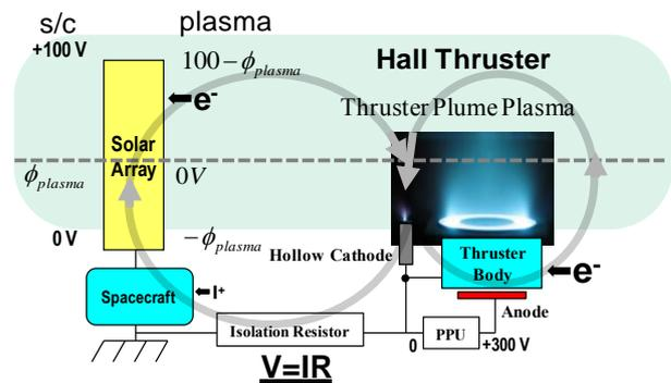
Figure 11. Current loops for Hall thruster with conducting pole pieces and thruster body at cathode common
