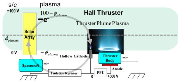
Figure 9. Cathode common circuit for a Hall thruster with insulating pole piece surfaces
