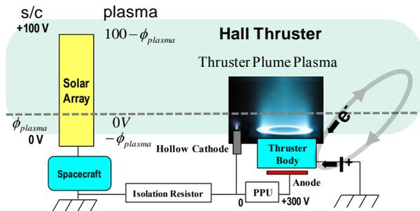
Figure 10. With conducting pole pieces current loop through thruster body closes in the plume plasma
