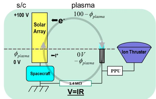
Figure 4. Electrons collected by the Dawn solar arrays cause a voltage drop across the isolation resistor
