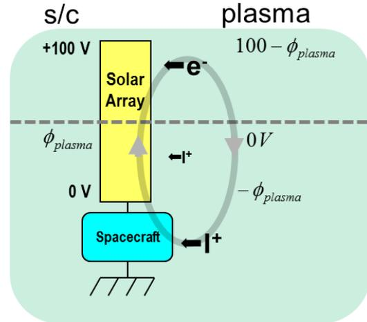
Figure 1. Spacecraft floating potential where ion current to the chassis balances electron collection to the solar arrays
