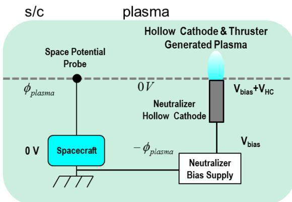
Figure 3. Potential in a hollow cathode produced plasma is about 15 V positive of cathode common
