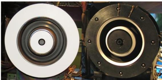
Figure 7 Hall thruster with insulating pole piece surfaces (left) and conducting surfaces (right).
