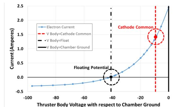
Figure 8. Hall thruster body electron currents with conducting pole pieces.
