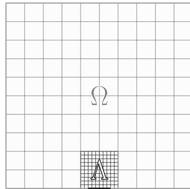
Figure 1. A localized patch  $\Lambda$  on a global mesh  $\Omega$ . Illustration on a structured 2D mesh.
