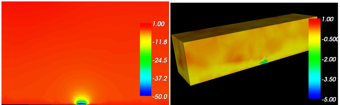
Figure 3. Resulting electrostatic potential around a  $-100$  V interconnect – Closeup on the interconnect and global solution
