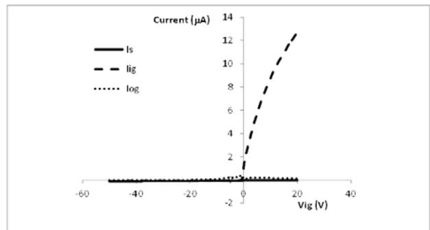
Figure 5: Current measured in RPA ion mode on the core sphere (Is), the inner grid (dashed line), and the outer grid (dotted line) as a function of the potential of the inner grid.
