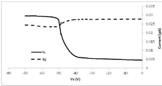
Figure 3: Current measured on the core sphere (solid line) and the inner grid (dashed line) as a function of the core sphere potential in EUV measurement mode.
