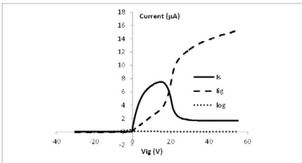
Figure 4: Current measured in RPA electron mode on the core sphere (Is), the inner grid (dashed line), and the outer grid (dotted line) as a function of the potential of the inner grid.
