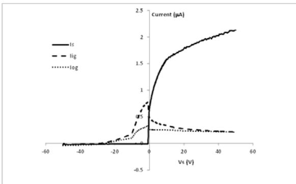
Figure 7: Current measured in Shielded Langmuir mode on the core sphere (solid line), the inner grid (dashed line), and the outer grid (dotted line) as a function of the potential of the core sphere.
