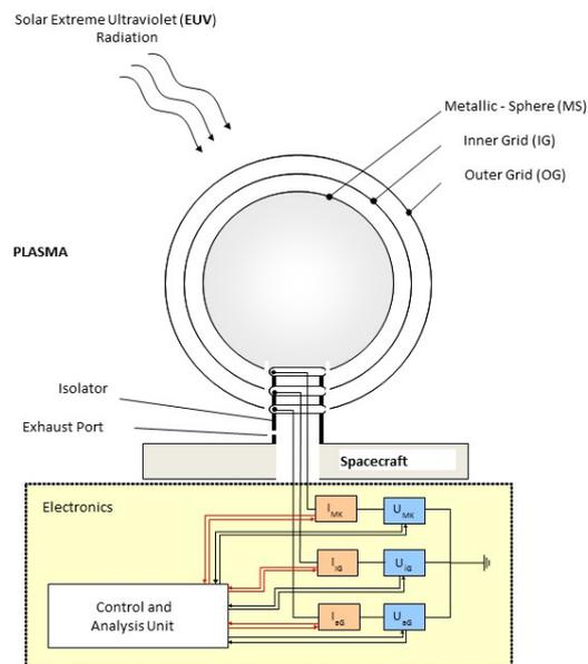
Figure 1: SEPS design. Each sphere is linked to its own electrometer and hence its own electronic circuit in charge of the control of the instrument and data processing.
