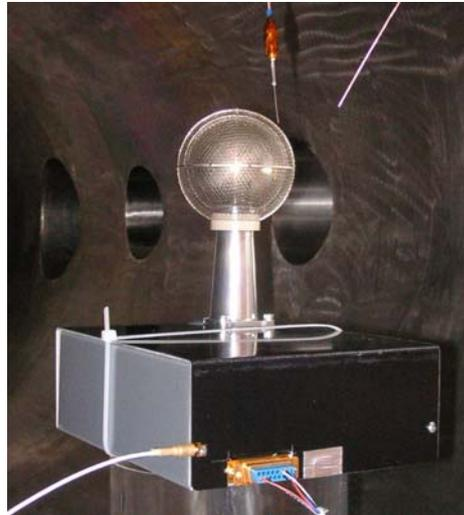
Figure 2: SEPS and the wire Langmuir probe in a plasma chamber at ESTEC.
