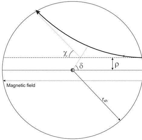
Fig. 5. Ion scattering under the action of the potential generated by a single tether. For symmetry consideration of the ion trajectory in a central field, the deflection angle  $\chi$  is equal to  $\pi+2\delta$ .
