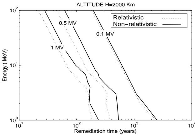
Fig. 8. Remediation time for a single tether moving at given altitude  $H=2000$  km for  $R=1$  mm,  $\phi_p=0.1, 0.5$  and  $1$  MV.
