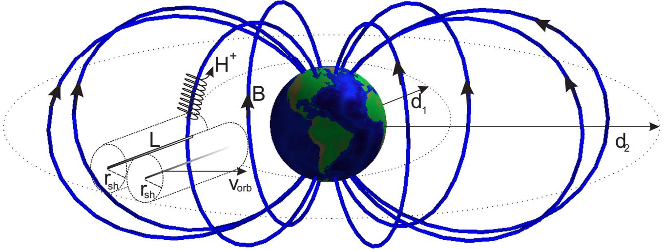
Fig. 1. Description of a vertical, electrostatic tether of length  $L$  moving in an equatorial, circular, direct orbit at given altitude  $H=(d_1+d_2)/2$ . Trapped, charged particles move helicoidally following Earth's magnetic field lines, bouncing back and forth. Several tethers should be considered for faster remediation; two tethers are also shown in the figure.
