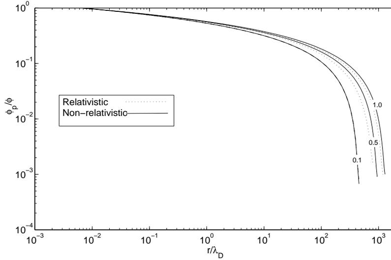
Fig. 3. Relativistic and non-relativistic potential profiles at  $H=2000$  km for  $R=1$  mm and  $\phi_p = 0.1, 0.5$  and  $1$  MV. For  $\phi_p = 0.1$  MV the sheath range is similar for both relativistic and non-relativistic model, whereas the relativistic model modifies the potential structure and reduce the sheath range for larger potentials.
