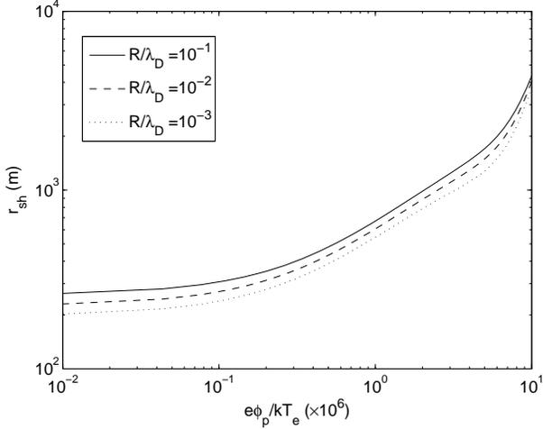
Fig. 4. Variation of the sheath range with the ratio  $e\phi_p/kT_e$  for several ratios  $R/\lambda_D$ .
