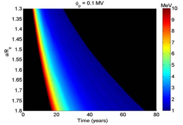
Fig. 9. Remediation time for the relativistic model. Considering 100 tethers moving in the same orbit for  $L=10$  km,  $R=1$  mm and  $\phi_p=0.1$  MV.
