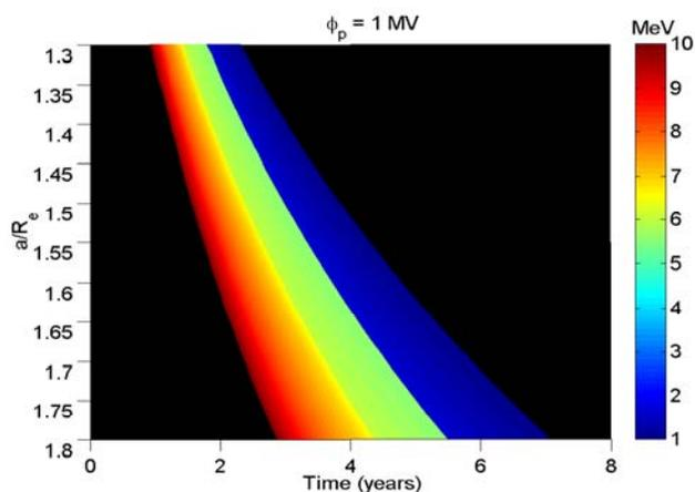
Fig. 11. Remediation time for the relativistic model. Considering 100 tethers moving in the same orbit for  $L=10$  km,  $R=1$  mm and  $\phi_p = 1$  MV.
