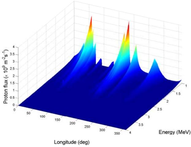
Fig. 7. Proton fluxes at  $H=2000$  km for a range of energies and orbital longitudes.
