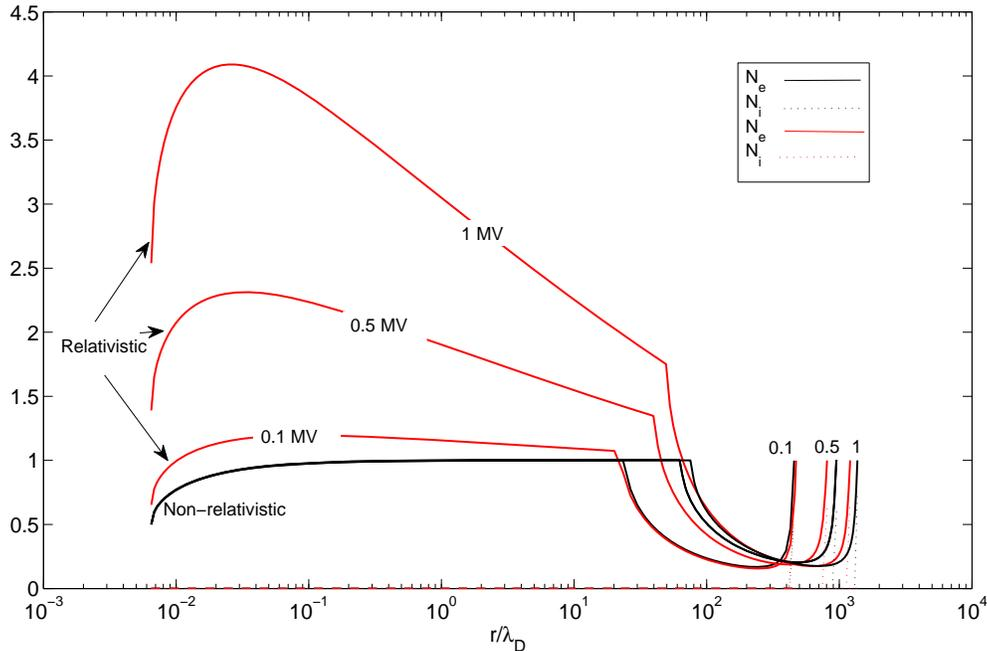
Fig. 2. Relativistic and non-relativistic density profiles at  $H=2000$  km for  $R=1$  mm and  $\phi_p = 0.1, 0.5$  and 1 MV. For a broad initial range the relativistic model larger  $N_e$  values. Notice that  $N_e \equiv n_e/n_\infty$  and  $N_i \equiv n_i/n_\infty$ .
