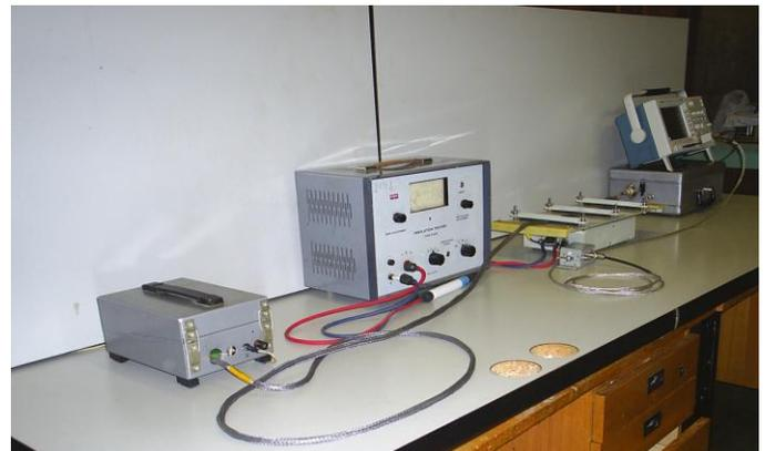
Fig.3. An experimental set-up intended for determining transformation coefficients converting ESD-induced structure currents into pulse voltages generated in cable harnesses. From left to right: a left set of equivalent load resistors for a cable to be tested, high voltage pulse generator, metal plate to provide an appropriate pulse current, a right set of equivalent load resistors for a cable and a Tektronix 3032B oscilloscope.
