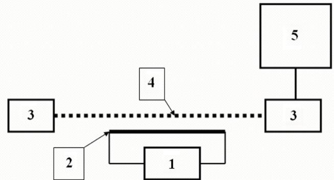
Fig.2. Block diagram of the experimental set-up for testing SC electrical cable harnesses. 1 – pulse current driver; 2 – metallic plate supporting the current; 3 – equivalent load resistor in shielded cable; 4 – harness fragment to be tested; 5 – Tektronix 3032B oscilloscope. Peak discharge current – (10...100) A; pulse length – (30...150) ns; pulse rise time – (3...5) ns; discharge energy – (0,02...0,2) J.
