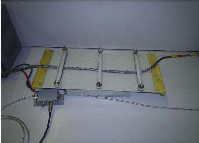
Fig.4. Experimental table, which is effectively a metallic plate to pass a pulse current. A cable harness is tightly pressed to the plate by dielectric planks. A current driver is placed under the plate, which is fabricated from the same alloy as the SC structure.
