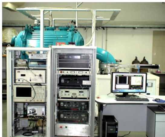
Figure 1: Experimental setup for testing arcing phenomenon on solar coupons
