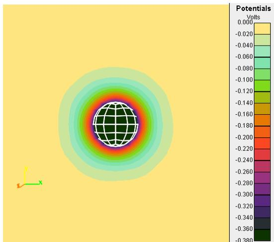
Fig. 6. Potentials in a plane through the center of a sphere computed using the Hybrid PIC method with better velocity resolution at the floating potential of  $-0.40$  V in a  $10^{11} \text{ m}^{-3}$ ,  $0.1$  eV plasma.
