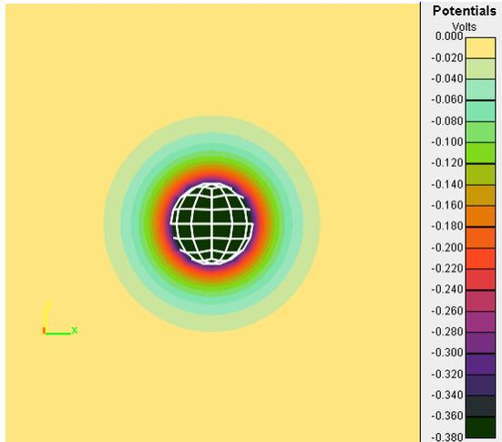
Fig. 4. Potentials in a plane through the center of a sphere computed using the analytic space charge density of (5) at the floating potential of  $-0.37$  V in a  $10^{11} \text{ m}^{-3}$ ,  $0.1$  eV plasma.
