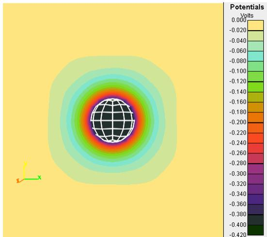
Fig. 5. Potentials in a plane through the center of a sphere computed using the Hybrid PIC method with minimal velocity resolution at the floating potential of  $-0.40$  V in a  $10^{11} \text{ m}^{-3}$ ,  $0.1$  eV plasma.
