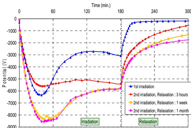
Fig. 8. Evolution of charging surface potential on FEP under successive irradiations with ( $20 \text{ keV}, 250 \text{ pA.cm}^{-2} + 400 \text{ keV}, 50 \text{ pA.cm}^{-2}$ ) and variation of relaxation duration between both irradiations : 3 hours, 1 week or 1 month
