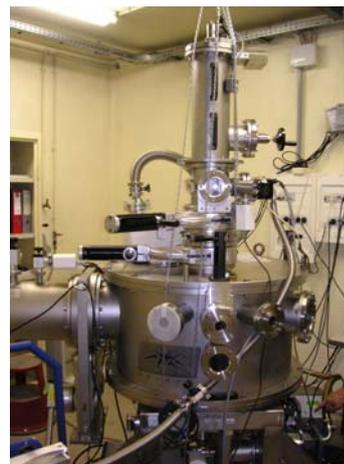
Fig. 4. SPIDER facility and its transfer unit STRASS installed on top.
