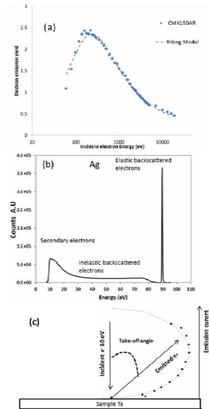
Fig. 10. Typical experimental results obtained in DEESSE and CELESTE. (a) Total electron emission yield measured on CMX150 AR. (b) Energy distribution of electron emitted from silver sample irradiated at 90 eV and biased at -9 V. (c) angular distribution of emitted electrons from tantalum sample irradiated at 60 eV at normal incidence.
