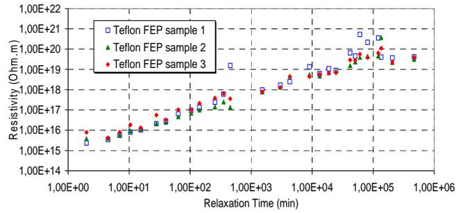
Fig. 7. Evolution of the apparent intrinsic bulk resistivity assessed on Teflon FEP samples
