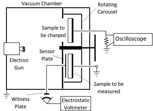
Figure 1. Electron gun and sample measurement system
