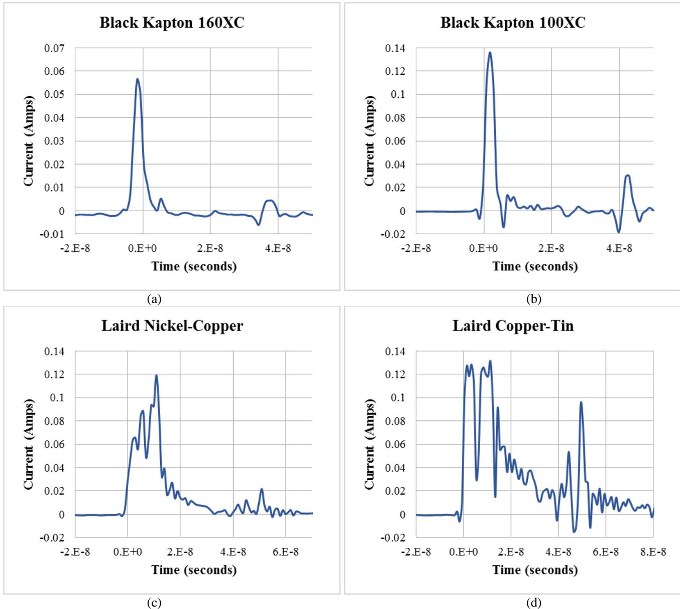
Figure 3. Largest discharges for all four conductive tapes
