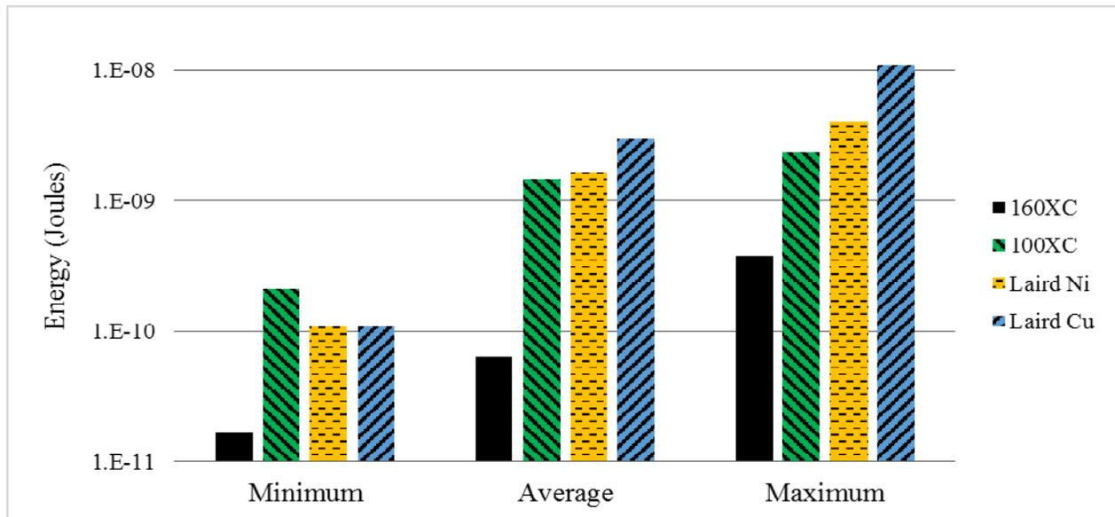
Figure 2. Discharge energy for four conductive tapes
